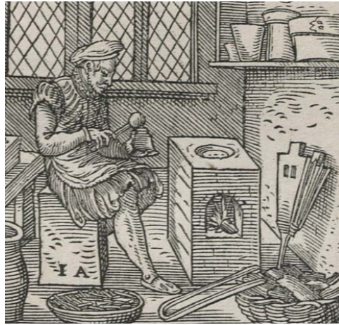
Image: 1568 illustration of a German type founder pouring type metal into a hand mold (Wikipedia).
